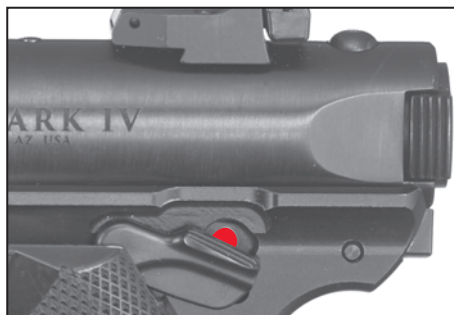
Figure 4. Safety in the “off” or “fire” position. Safety is all the way down and red dot is visible.
